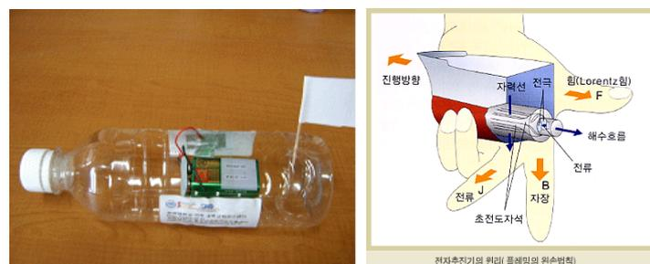
Figure 1. Lorentz ship: a simplified model (left) and a force diagram (right)
