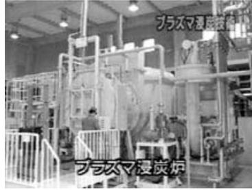
Carbon coating on steel by plasma (Shimane Pref.)
