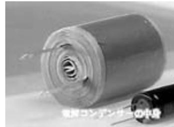
Separator for electrodeposited capacitor
